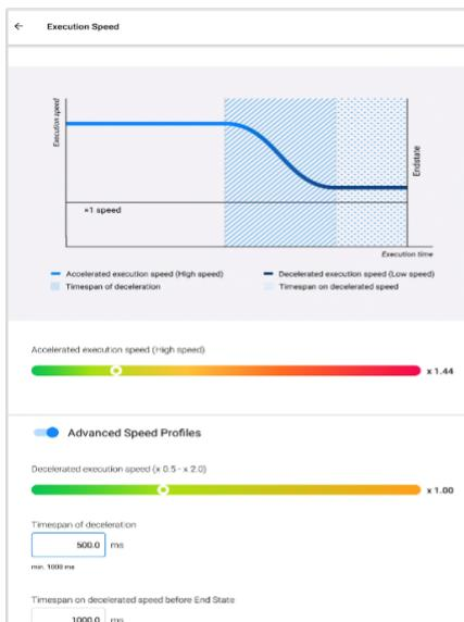
④ Select the **Advanced speed profiles** checkbox to **proceed to the advanced settings**.
